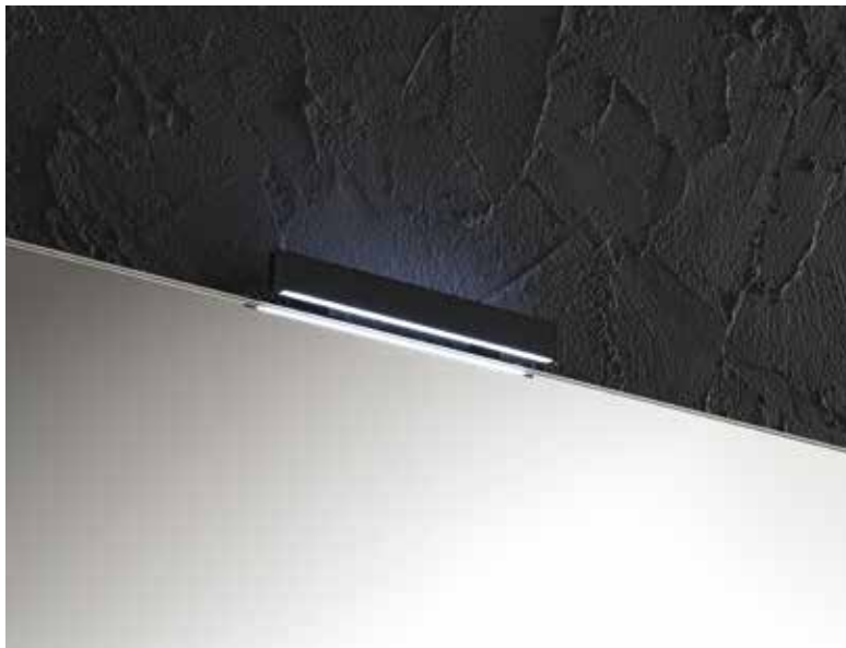
FA343 - FA344 DUAL lamp, Matt black (343) or white (344) Dimensions: 40x4x4H cm LED 13,4Watt 12 V with trasformer 4000K° IP44
